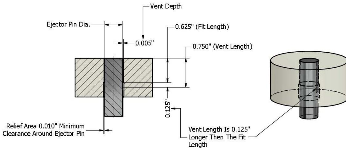
Something that is often overlooked in venting is the polish. It is recommended that all vents be **draw polished** in the direction of flow to at **least** the same finish as the cavities and cores. They should be polished for their entire length including the relieved distance. If a mold is to be chrome plated, all the **molding surfaces** should be polished and plated including the vents.
